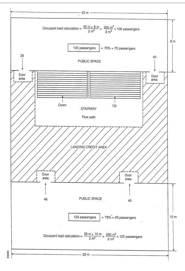
Figure 3 - Occupant loading calculation example
